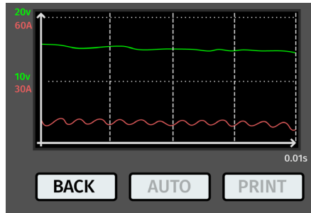
Figure 12. Diagram of the measured voltage and current of the diagnosed alternator.
