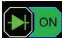
Figure 4. Display of the diode symbol on the tester screen
