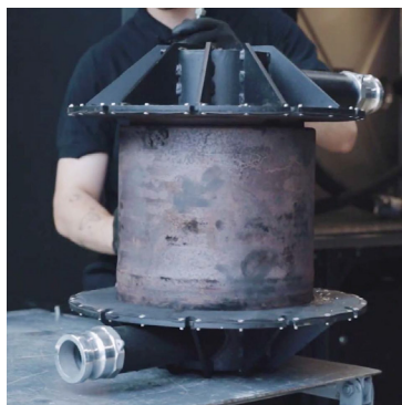
Figure 29. Mounting the fitting on the filter
