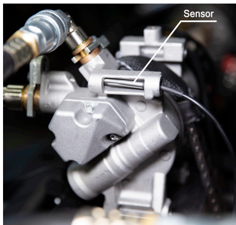
Figure 29. Position of a contact temperature sensor
