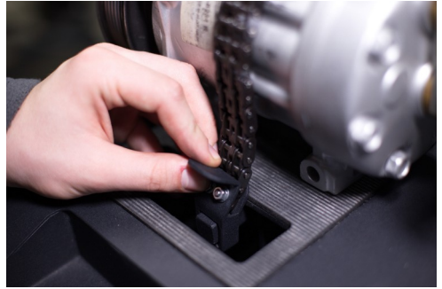
Figure 23. Mounting and fixing of a compressor on the Test Bench
