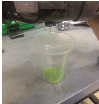
Figure 21. Monitoring of compressor oil condition
