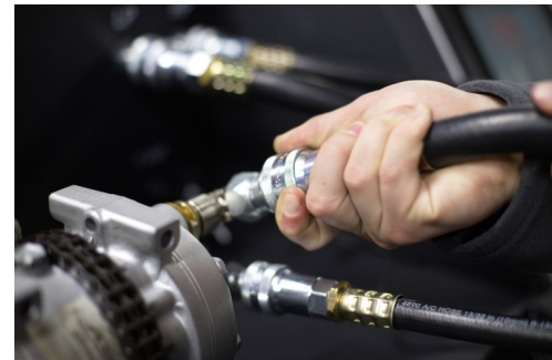
Figure 25. Connection of the LP and HP lines to a compressor
