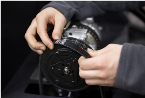
Figure 24. Adjusting the belt and checking its tightness
