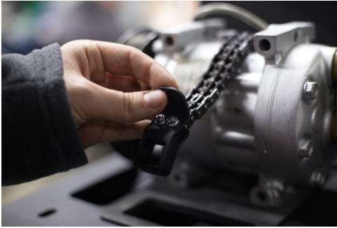
Figure 23. Mounting and fixing of a compressor on the Test Bench
